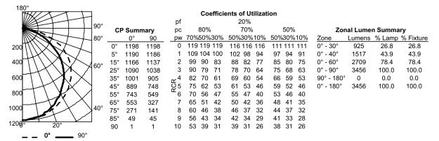
2AVL4 40L MDR LP835, 4255 delivered lumens, test no. 69071P5, tested in accordance to IESNA-LM79.
